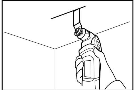
Put the application tool on the workpiece. And then move the tool forward so that the application tool movement does not slow down.
