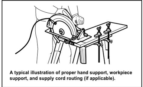
A typical illustration of proper hand support, workpiece support, and supply cord routing (if applicable).
