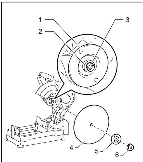
► 1. Inner flange 2. Ring 3. O-ring 4. Cut-off wheel
