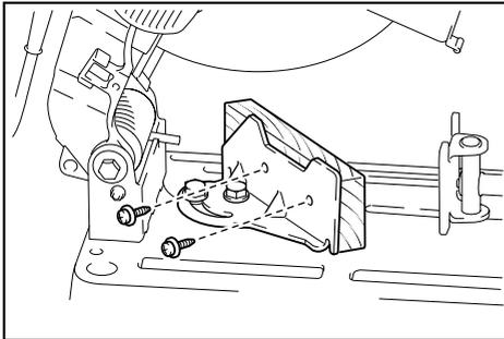
When the cut-off wheel has worn down, raise the cutting position by putting a spacer block which is slightly narrower than the workpiece as shown in the figure. This will help you to utilize the wheel economically.
