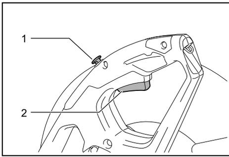
► 1. Lock button / Lock-off button 2. Switch trigger
