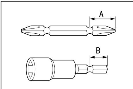
Use only driver bit/socket bit that has inserting portion shown in the figure. Do not use any other driver bit/socket bit.
