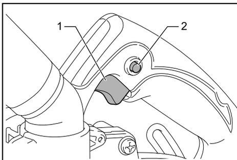
► 1. Switch trigger 2. Lock button / Lock-off button
