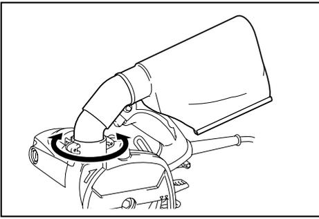
When the dust bag is about one-third full, remove the dust bag from the tool and pull the fastener out. Empty the dust bag of its contents, tapping it lightly so as to remove particles adhering to the insides which might hamper collection.
