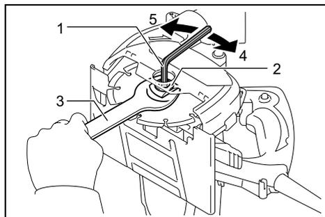
► 1. Hex wrench 2. Hex bolt 3. Wrench 22 4. Loosen 5. Tighten
